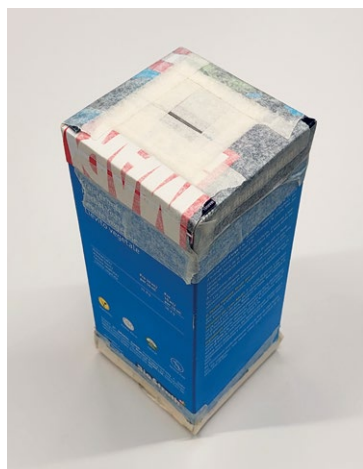
DIY spectrometer: incoming light is collimated (made parallel) through a slit consisting of two razor blades and spectrally split at the other end by a CD acting as a diffraction grating. Students can use the angle of diffraction to determine the wavelengths of light from various sources.
